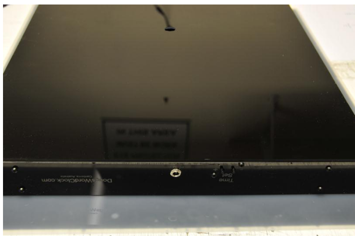
Rear view of a 50cm WordClock showing low voltage power socket and time setting buttons.
